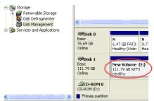
If you are installing a hard drive that already has data on it, then after plugging it in, the drive should automatically show up with a drive letter assigned within "My Computer". You can verify or change the drive letter through Disk Management, as outlined above.
